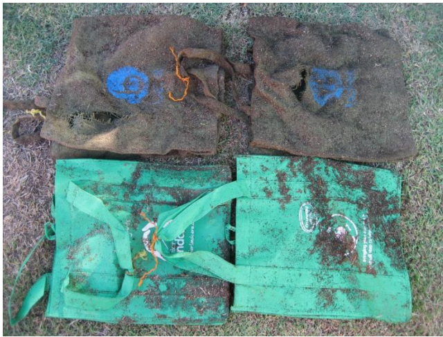
Figure 2. Bebak bags could be ripped apart compared to ‘green bags’ which remained intact after 7 days of composting
