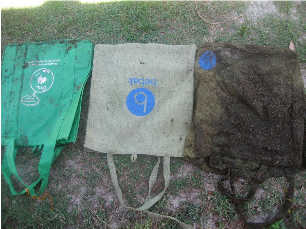
Figure 3. The bebak bags in the compost has started degrading fast (right) compared to that left in the garden (middle) and the 'green bags' (left) after 14 days
