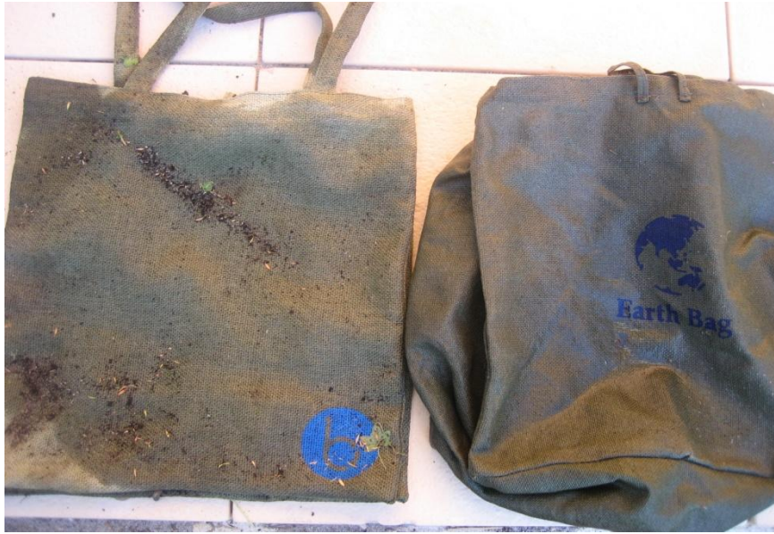
Figure 6. The bag left in the garden (left) and immersed in water(right) after 28 days
